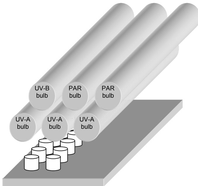
**Figure 1:** Schematic diagram of the experimental apparatus, showing the arrangement of the bulbs and the placement of the experimental dishes (not to scale). Three apparatuses, each containing 20 dishes, were used in each trial.
